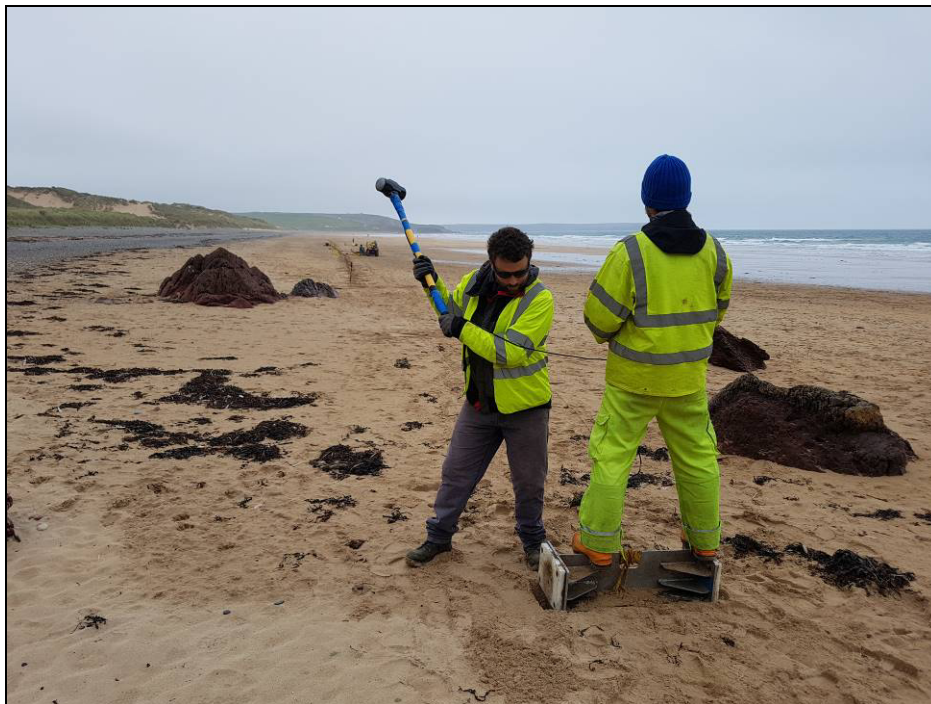
Plate 8 – S-wave survey being carried out at Freshwater West site.
