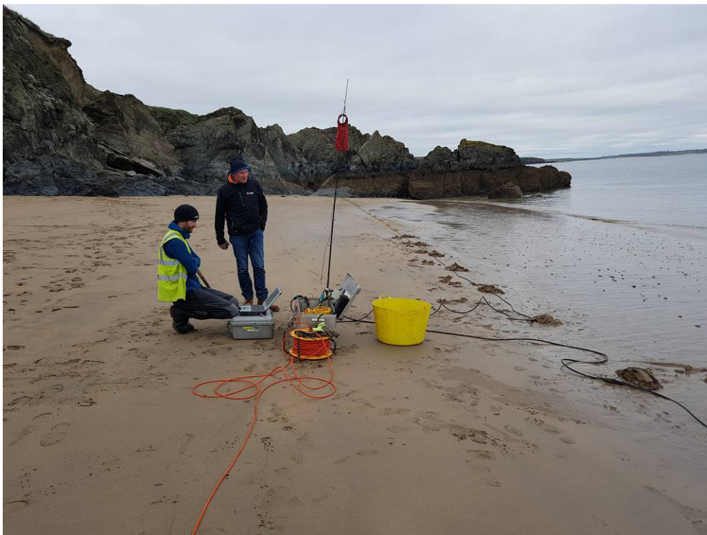
Plate 7 – Seismic recording set-up on Profile 4
